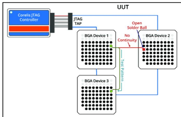
***Faults can be diagnosed to a single pin with three interconnected BGA boundary scan devices.***
