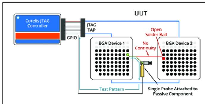
***BGA open faults can be diagnosed to a single pin using a combination of JTAG and a GPIO pin.***
