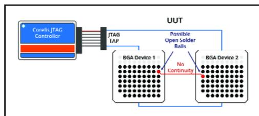
*JTAG testing can be used to identify faults between BGA boundary scan devices.*
