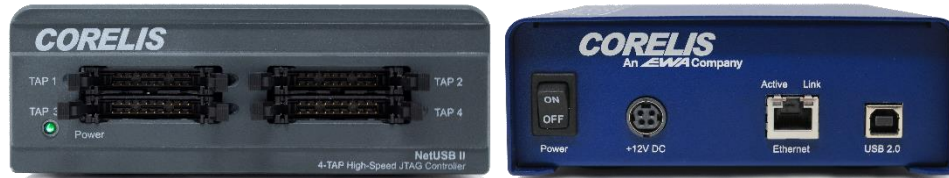
Figure 1-3. Net USB II 4-TAP front panel (left) and rear panel (right).
